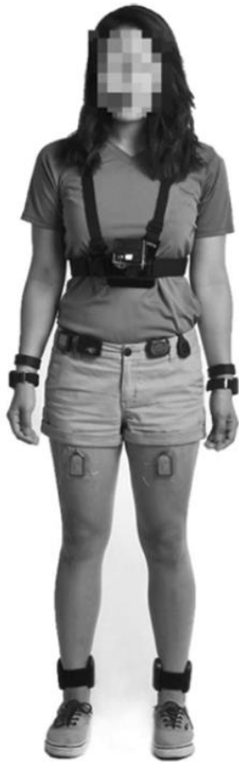
FIGURE 1—Placement of all devices on the body. Two SW devices on each ankle; one AP on each thigh; one AG, NL, DW, and FZ on the hip; one AG on each wrist; one FC on each wrist; and one GoPro camera worn on the chest.
